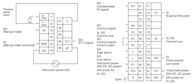
Note: \*Symbols for AC instrument power are VPO, PCO. Output: Approx. 24V DC (0.1A max.)
